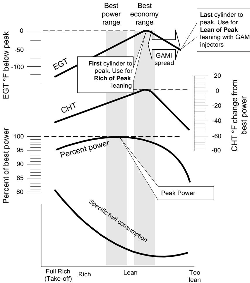
As the mixture is leaned, EGT rises to a peak temperature, and then drops as the mixture is further leaned. Peak *power* occurs at a mixture using more fuel than at peak EGT. Best *economy* occurs at peak EGT. Accurate leaning yields optimal engine temperatures. By being able to precisely adjust the mixture, your engine can produce either the best fuel economy or maximum power, whichever you choose.
