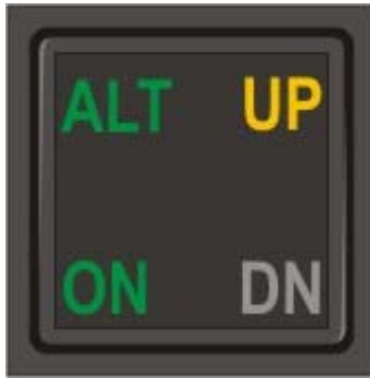
Fig. 2-29. ALT HOLD ON/OFF Switch Display, ALT HOLD Mode Engaged, TRIM UP Required (System Thirty ALT)
