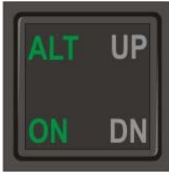
Fig. 3-6. ALT HOLD ON/OFF Switch Display, ALT HOLD Mode Engaged (System Thirty ALT)
